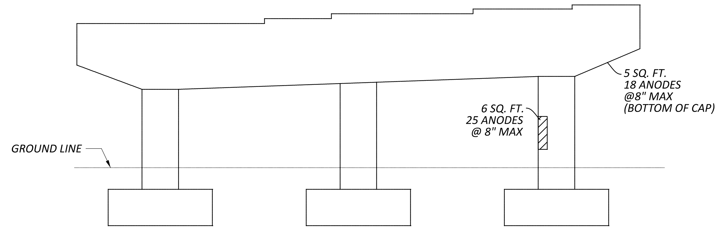
PIER 9N - WEST ELEVATION (LOOKING EAST)
