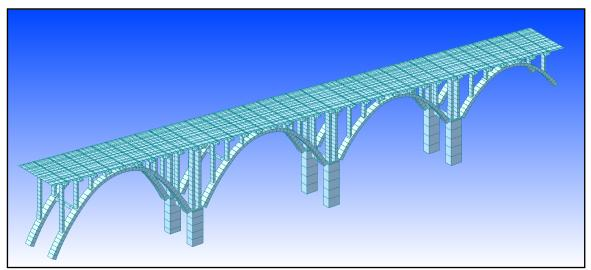
Figure E. Isometric View of Arch Spans' 3D Model
