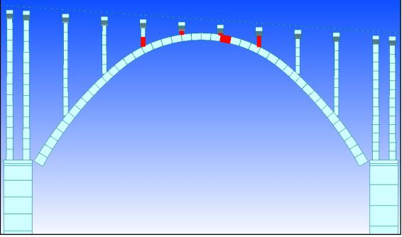
Figure J. Arch Span B with cracked arch rib and spandrel column elements in red
