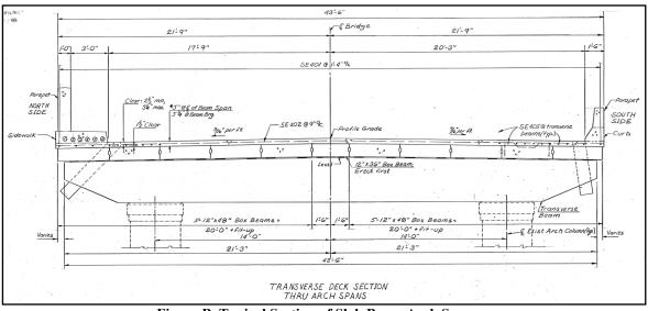
Figure B. Typical Section of Slab Beam Arch Spans
