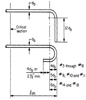
Figure C5.10.8.2.4a-1—Hooked Bar Details for Development of Standard Hooks (ACI Committee 318 2011)
