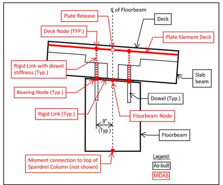
Figure D. Elevation View of Deck to Floorbeam Connection
