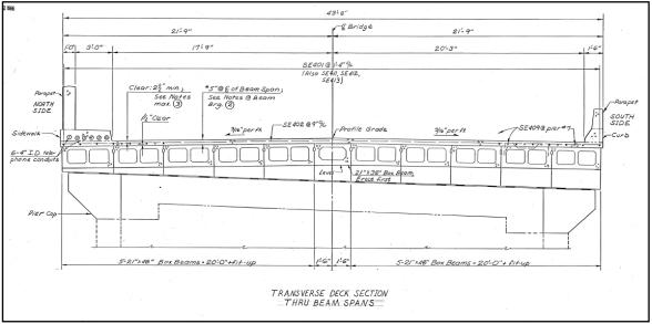
Figure A. Typical Section of Box Beam Approach Spans
